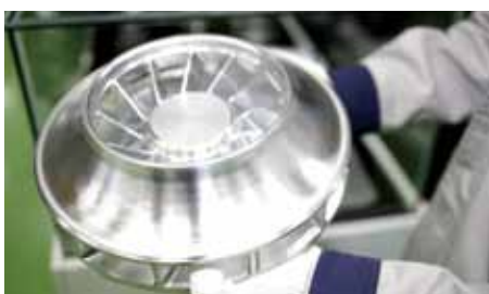
➤ A blocked type of impeller that can only be processed through simultaneous 5-axis operations.
