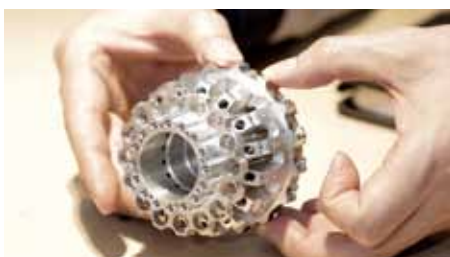
➤ The result of split 5-axis machining, where one side is machined and then the rotating shaft is rotated for machining of the next side, as described by Jang Dong Sik, a manager of Doosan Machine Tools.
