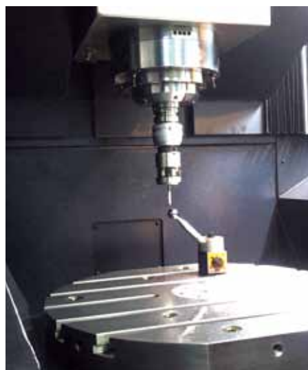
➤ Rotation center axis correction work being carried out by the IKC solution used alongside the calibration software and hardware consisting of a touch probe, a datum ball, an automatic tool length measuring device, and a master tool.
