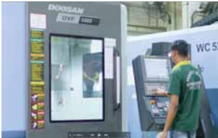
➔ Perfect Team Engineering is using a 5-axis machining center to machine parts for the oil & gas industry.
