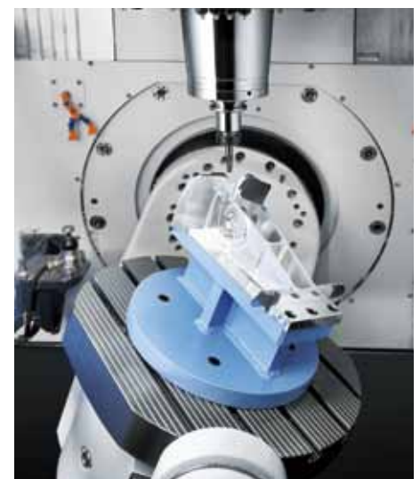
➤ The DVF 5000 in operation. The simultaneous 5-axis equipment can also support split 5-axis operations, whereas the split 5-axis machining center does not support simultaneous operations. Choose the type of equipment according to your specific machining needs.
