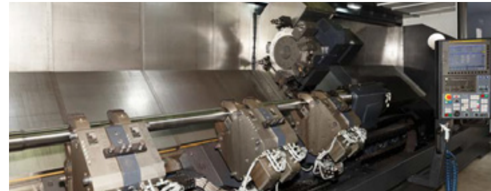
ⓘ Six cradles prevent vibration by supporting a long shaft. Hetraco plans to introduce more PUMA 700XLY.
