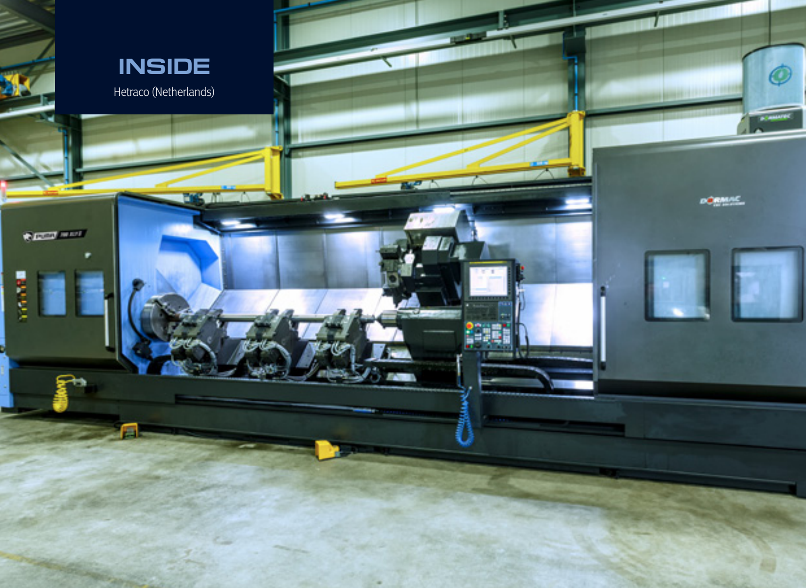
ⓘ DN Solutions' PUMA 700XLY, newly introduced by Hetraco, has a machining length of 5m and 6 steady rests.
